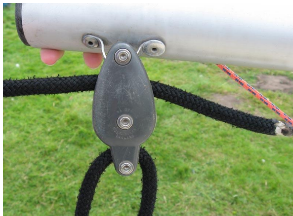
Picture 2.13 Through the boom end block
