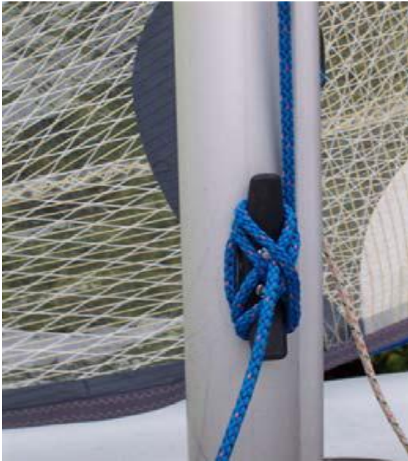
Picture 3.3 The jib halyard cleat
