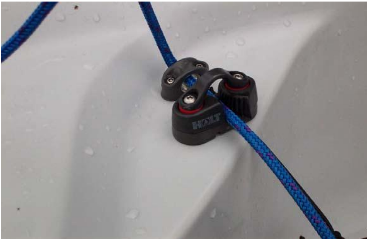
Picture 3.3 The bulls eye and jib cleat
