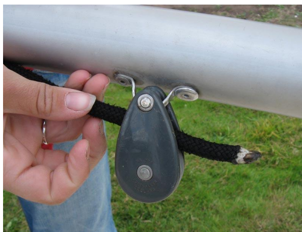
Picture 2.15 Through the middle boom block
