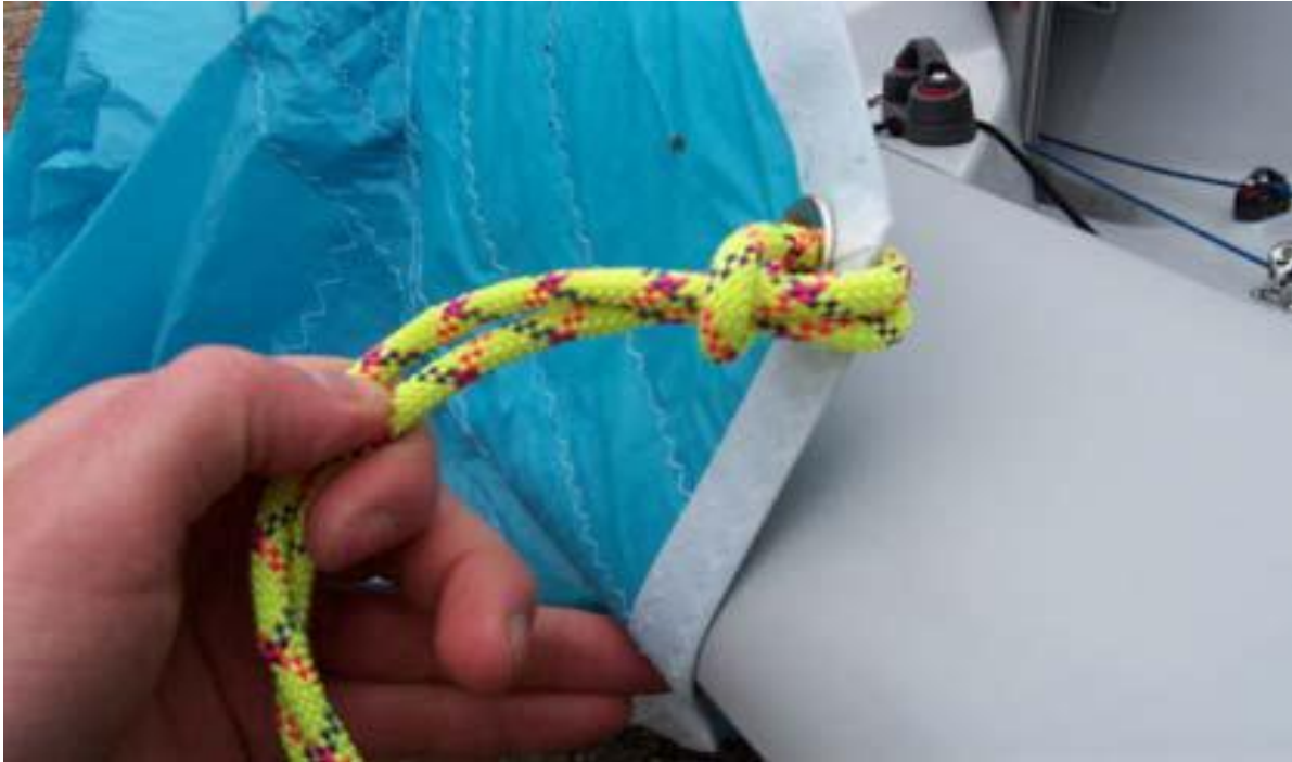
Picture 4.4 Tying the Spinnaker Sheets
