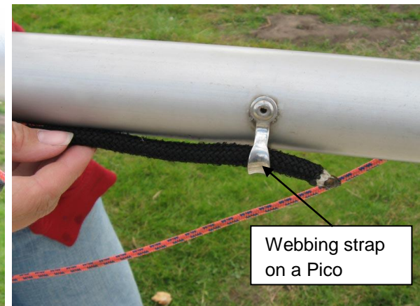
Picture 3.6 Through eyehole on boom
