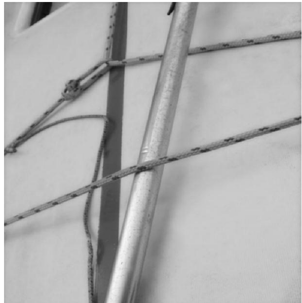
Picture 3.16 Tiller UNDER the traveller
