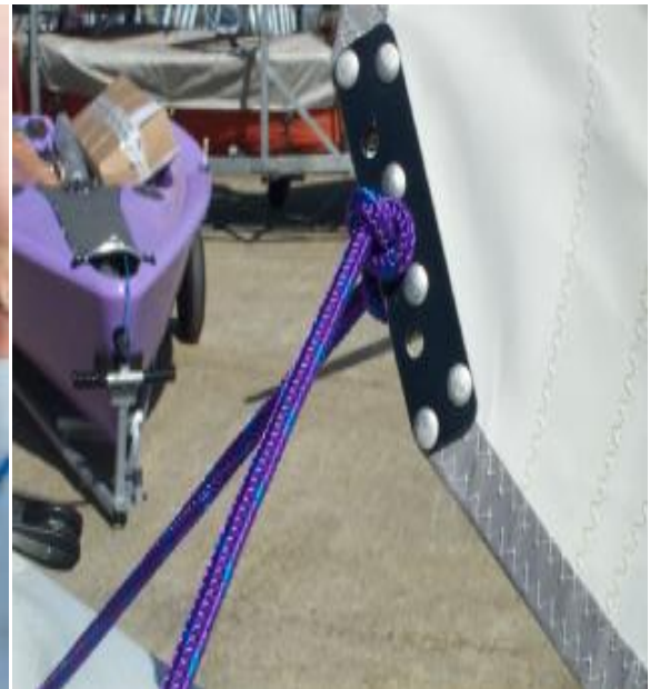
Picture 3.4 The jib sheet connected
