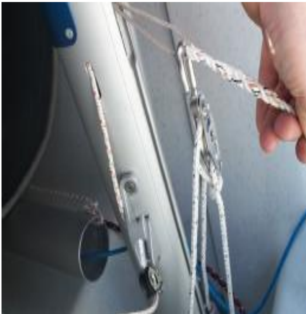
Picture 3.3 Connecting the rig tension.
